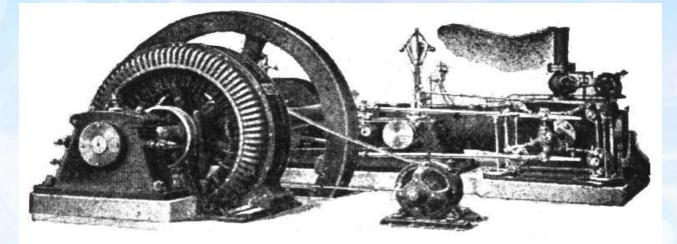
The Dynamo was the first electrical generator capable of delivering power for industry. The dynamo uses electromagnetic principles to convert mechanical rotation into a pulsing direct electric current through the use of a commutator. A dynamo machine consists of a stationary structure, which provides a constant magnetic field, and a set of rotating windings which turn within that field.
