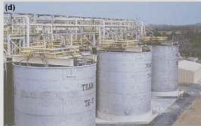
Commercial Bioleaching Tanks
