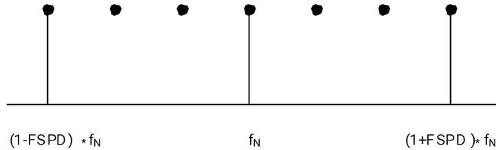
**Figure 1. Frequency Spread Definition**
