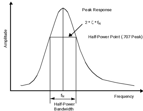
Figure 2. Half-Power Bandwidth Definition
