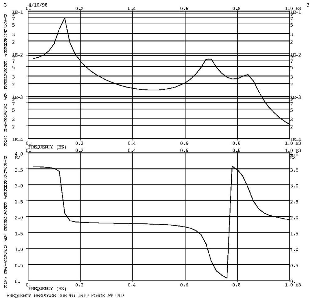
FREQUENCY RESPONSE DUE TO UNIT FORCE AT T1P
