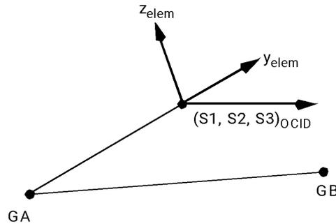
Note: 1. The material stiffness and damping properties of the elastomer are located at (S1, S2, S3).
