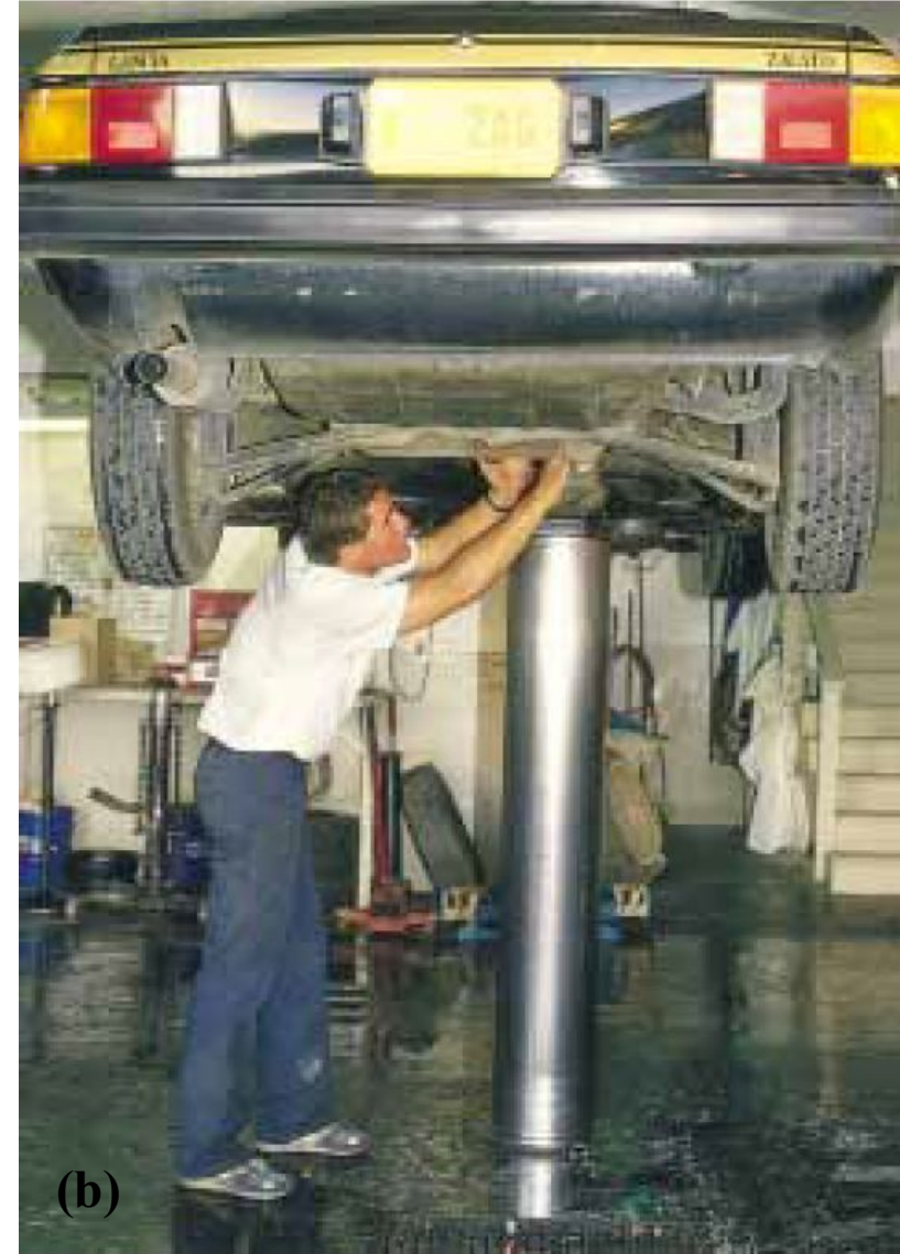
Figure 7.4 (a) Diagram of a hydraulic press. Because the increase in pressure is the same on the two sides, a small force F_1 at the left produces a much greater force F_2 at the right. (b) A vehicle undergoing repair is supported by a hydraulic lift in a garage.
