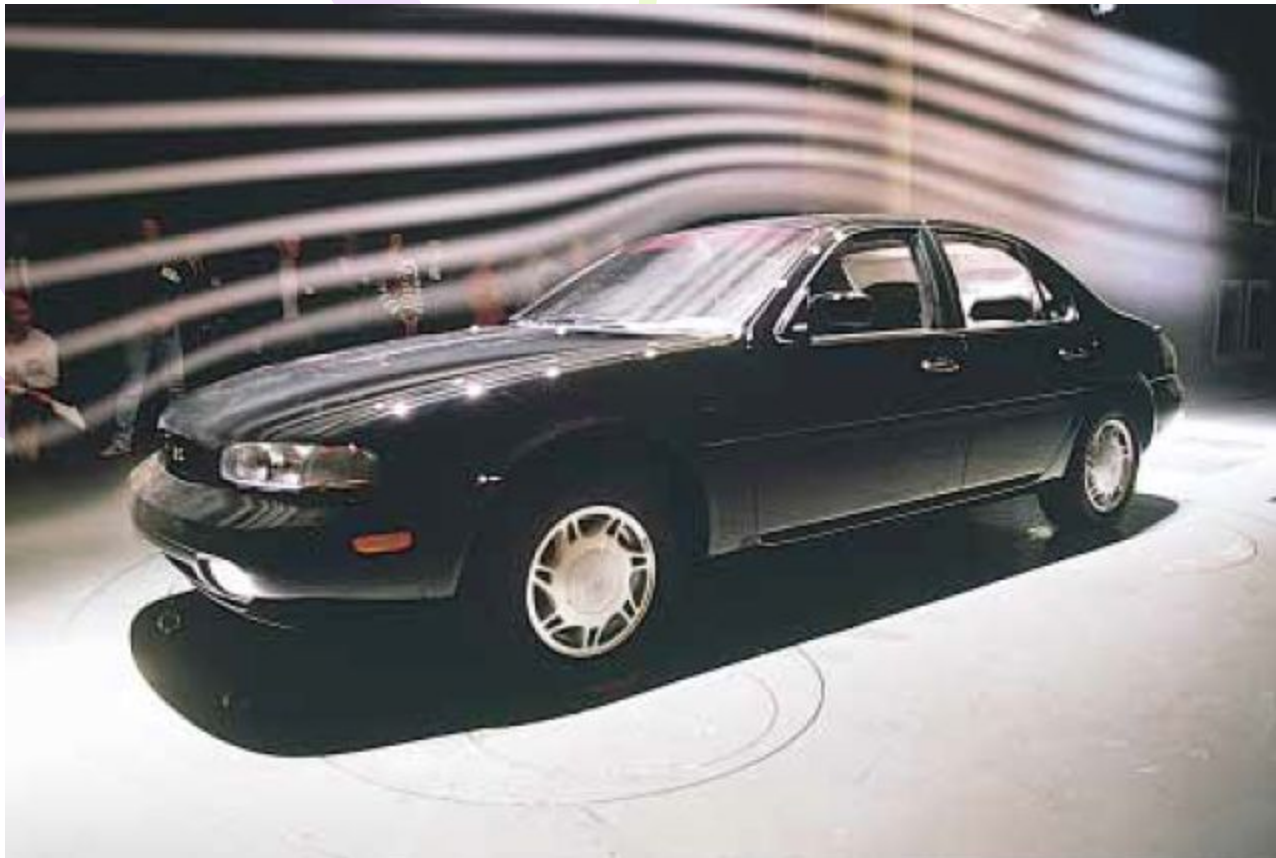
Figure 7.10 Laminar flow around an automobile in a test wind tunnel.
