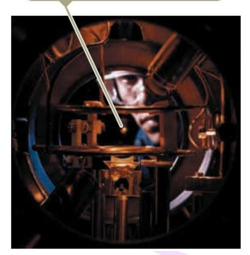
An extension of laser trapping, laser cooling, is possible because the normal high speeds of the atoms are reduced when they are restricted to the region of the trap. As a result, the temperature of the collection of atoms can be reduced to a few microkelvins. The technique of laser cooling allows scientists to study the behavior of atoms at extremely low temperatures
