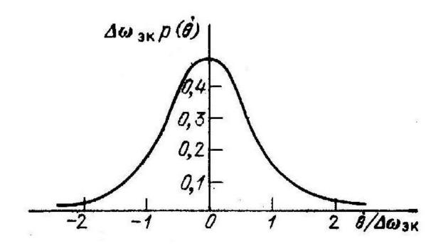
$$p(\dot{\theta}) = \left[ 2\Delta\omega_{\partial R} \left( 1 + \frac{\dot{\theta}^2}{(\Delta\omega_{\partial R})^2} \right)^{3/2} \right]^{-1}$$
