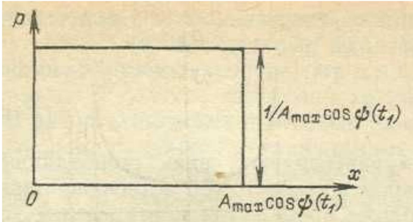
$$M\{x(t_1)\} = \frac{1}{A_{max} \cos \psi(t_1)} \int_0^{A_{max} \cos \psi(t_1)} x dx = \frac{1}{2} A_{max} \cos \psi(t_1)$$
