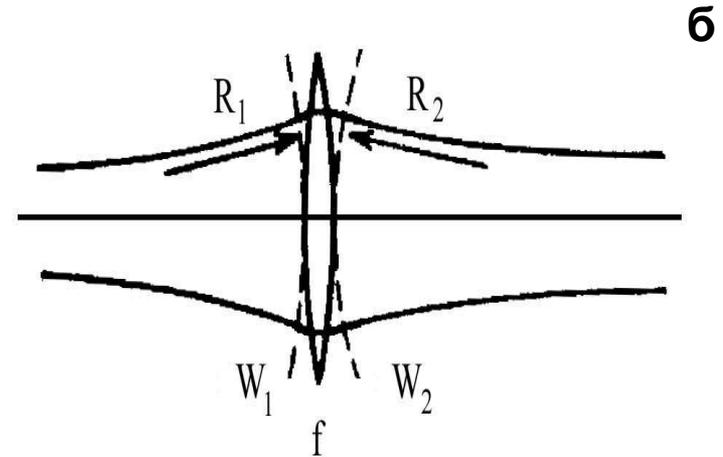
$$\frac{1}{R_2} = \frac{1}{R_1} - \frac{1}{f}, \quad W_1 = W_2, \quad -\frac{2i}{kW_1^2} = \frac{1}{q_1} - \frac{1}{R_1} = -\frac{2i}{kW_2^2} = \frac{1}{q_2} - \frac{1}{R_2}$$
