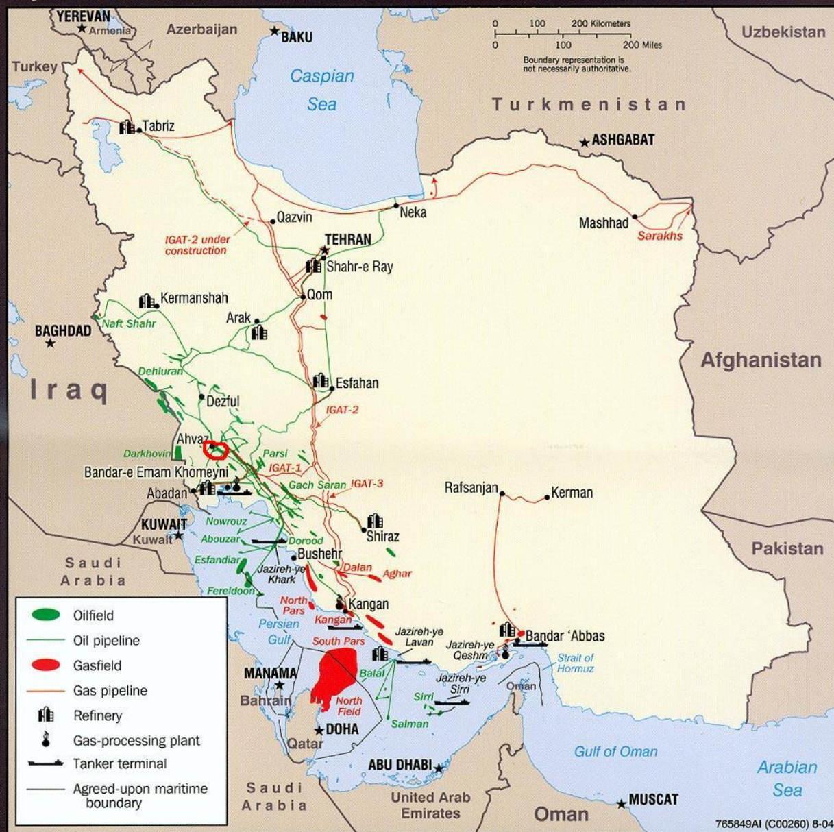
Key Petroleum Sector Facilities
