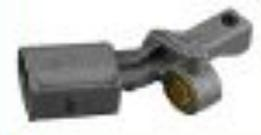
Lateral acceleration sensor and yawrate sensor (cluster)
