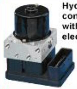
Hydraulic control unit with integrated electronic controller
