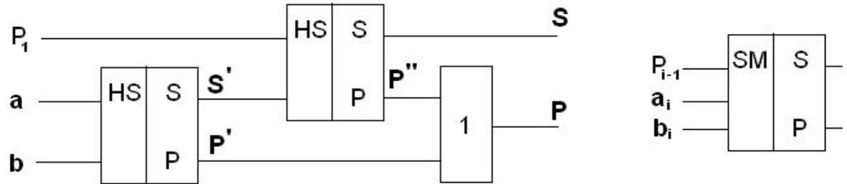
$$P'' = (a \oplus b)P_{-1}, \quad P = ab \vee (a \oplus b)P_{-1} = ab \vee (ab)(a \vee b)P_{-1} = ab \vee (a \vee b)P_{-1} = ab \vee aP_{-1} \vee bP_{-1}$$
