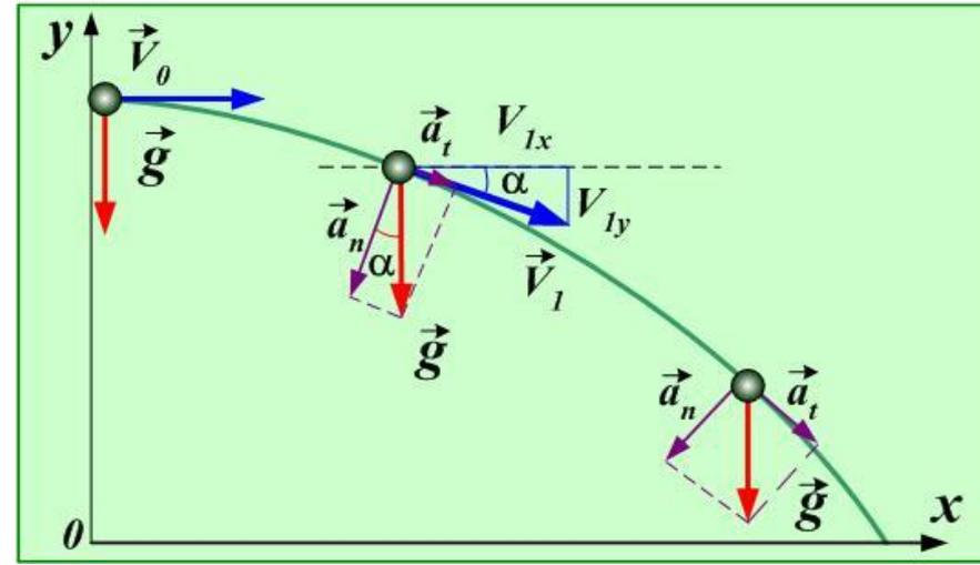
$$\frac{gv_0}{\sqrt{v_0^2 + g^2 t^2}} = \frac{(v_0^2 + g^2 t^2)}{R}.$$
