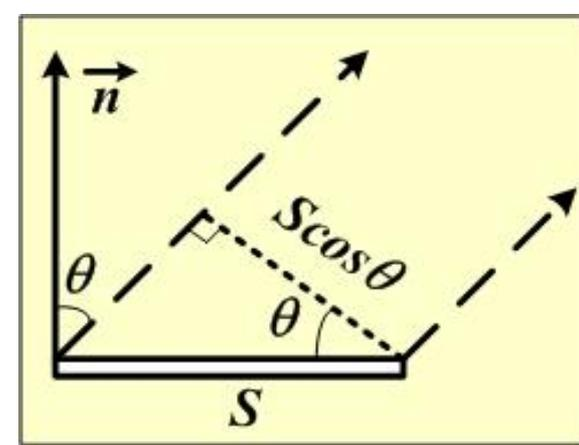
$$\Phi_v = \int_0^{2\pi} \int_0^{\pi/2} jS \cos \vartheta \sin \vartheta d\vartheta d\varphi = \frac{w_v c}{4\pi} S \int_0^{2\pi} \int_0^{\pi/2} \cos \vartheta \sin \vartheta d\vartheta d\varphi =$$
