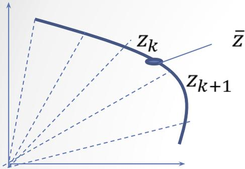
$$\begin{aligned} S_n &= \sum_{k=1}^n f(\bar{z}_k) \Delta z_k = \\ &= \sum_{k=1}^n (U(\bar{x}_k, \bar{y}_k) + iV(\bar{x}_k, \bar{y}_k))(\Delta x_k + i\Delta y_k) \\ \int f(z) dz &= \lim_{n \rightarrow \infty} S_n \end{aligned}$$
