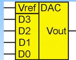
$$V_{out} \sim V_{ref} \times (\text{code})$$
