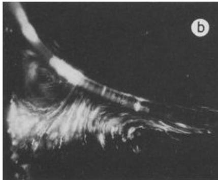
Fig. 4a, b. Experimental scheme for observing and recording motion of the liquid in laser-heated zone **a** and stream formation in the liquid towards free surface **b**
