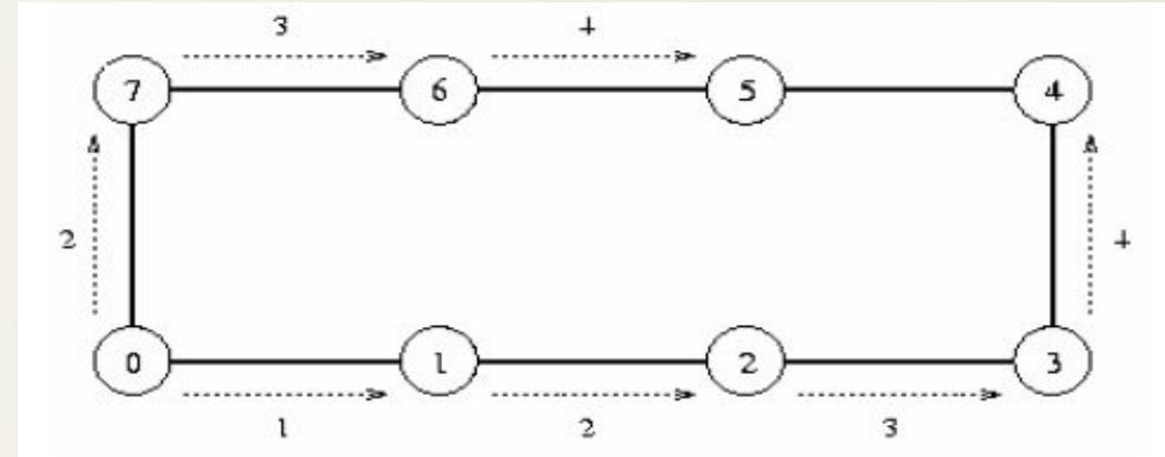
$$t_{nd} = \sum_{i=1}^{\log_2 p} (t_H + mt_K + t_c p / 2^i) = (t_H + mt_K) \log_2 p + t_c (p - 1)$$
