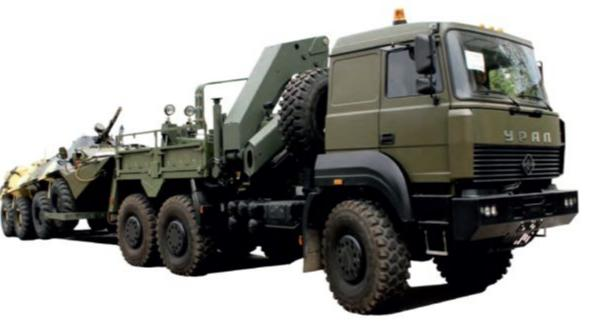
Wrecker is designed for support of convoy movement, recovery of damaged motor vehicles on all kinds of roads and terrain, rendering technical assistance, re-priming with fuel, lubricants and special fluids, loading and unloading of cargo.
