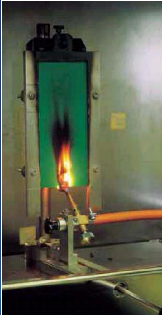
Example: Fire exposed to edge
