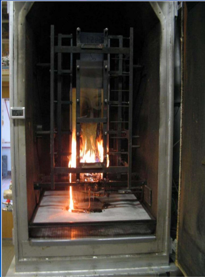
Ignition of glass clear PE panels: crossfall „burning droplets“
