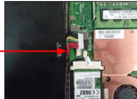
Remove key part before requirement remove battery connector for safety.
