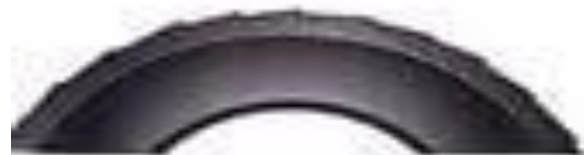
Diagonal Wear / Heel & Toe Wear
