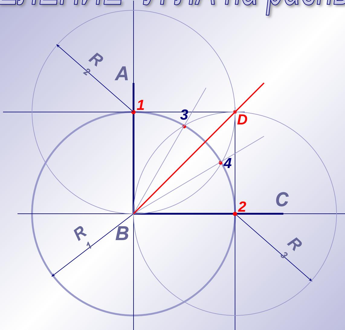
$$R_1 = R_2 = R_3$$
