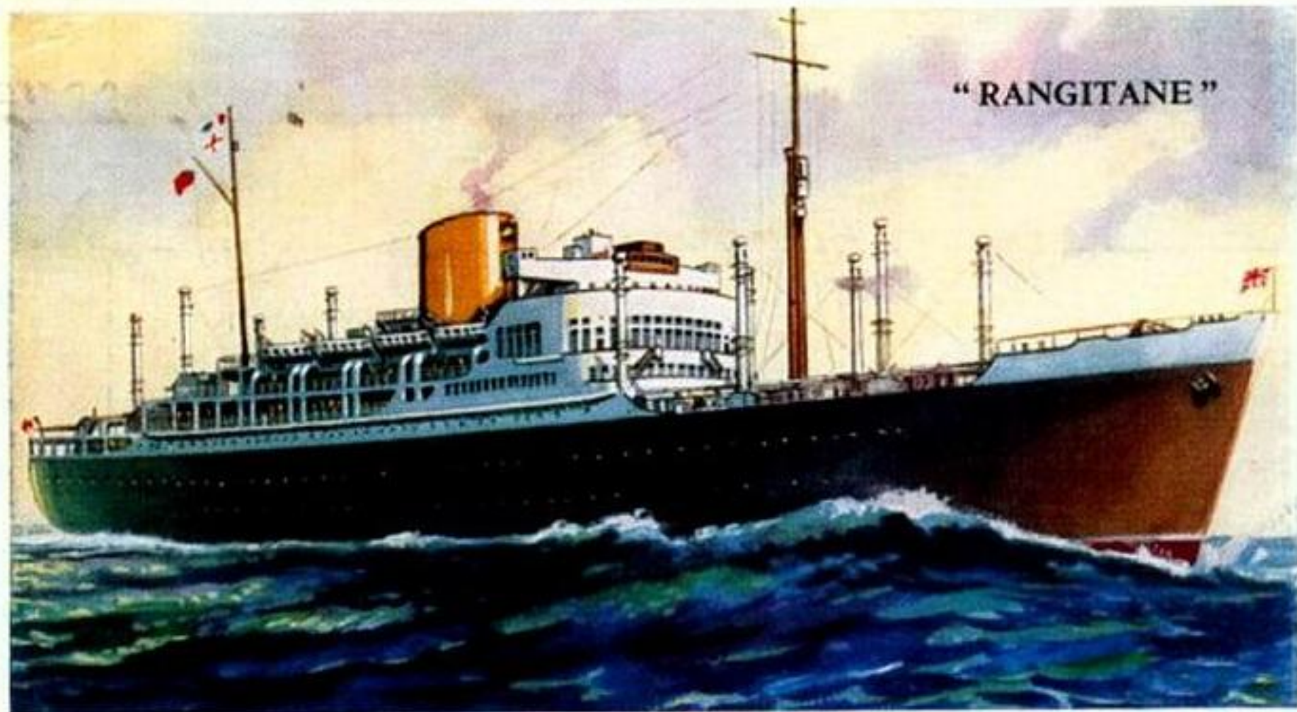
R.M.M.V. "Rangitane" — New Zealand Shipping Co. Built 1949 by John Brown & Co. Weight 21,868 tons; Service speed, 17 knots; Length, 609 ft.; Breadth, 81 ft. Passengers, 392 in one class. Sister ships are the "Rangitoto" and "Rangitiki."
