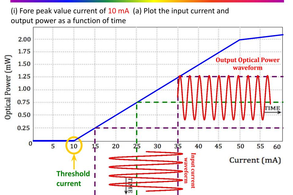
b) Does the laser behave as a linear device for this modulating current? Why?
