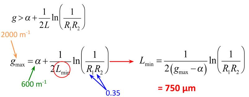
(ii) If the cavity length is required to be  $L = 475 \mu m$  and R1 = R2 = R, what is the minimum value for the reflector value R?
