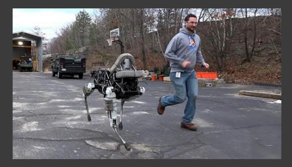
Spot is a four-legged robot designed for operations inside and outside. Electrically powered and hydraulically actuated, it sports a sensor so it can find its way around rough terrain.
