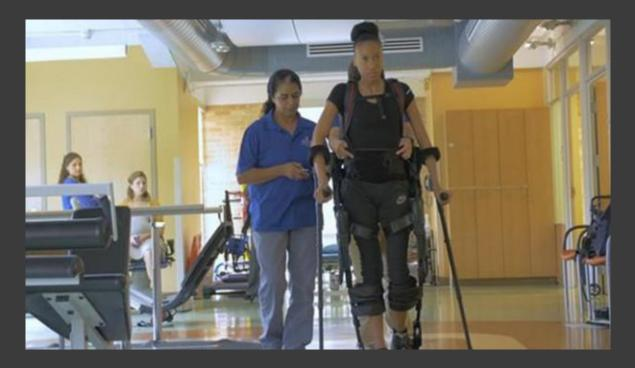
Its latest product, the Ekso GT, is helping spinal trauma and stroke victims recover and walk again. The robotic suit, made from titanium and aluminium, uses battery-powered motors to allow the wearer to walk. All they need to do is move their hips forward, and the device will initiate steps. It also comes with software that health professionals can use to provide adaptive therapy.
