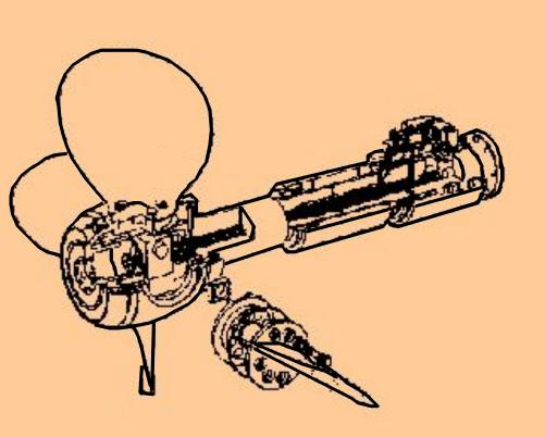
By changing the position of the blades the *propeller-pitch* can be controlled.
