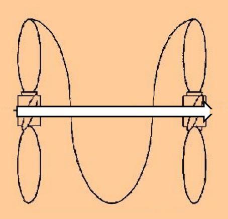
By *pitch* is understood the *distance travelled* after *one revolution* of the screw.
