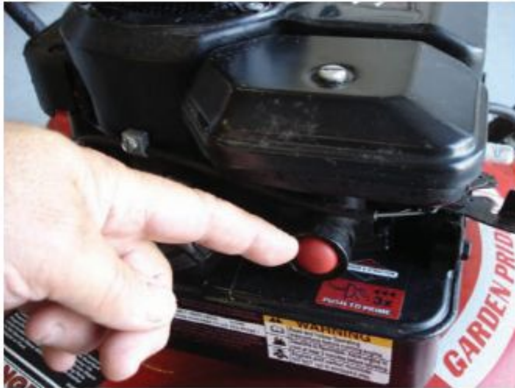
Figure 9 A primer cold start system pushes fuel directly into the engine.
