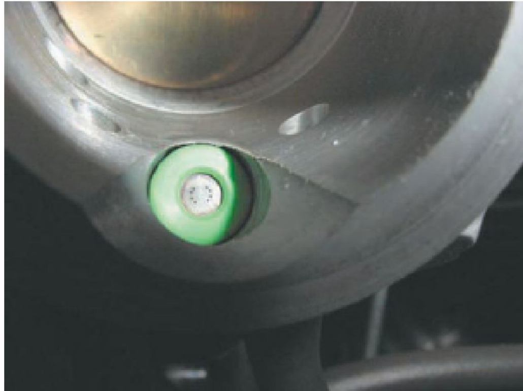
Figure 42 Various types of tips can be found on a fuel injector. Decisions on the type of injector to be used can be based on intended use as well as cost.
