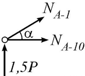
$$\begin{aligned}\Sigma X &= N_{A-10} + N_{A-1} \cos\alpha = 0; \\ \Sigma Y &= N_{A-1} \sin\alpha + 1,5P = 0.\end{aligned}$$
