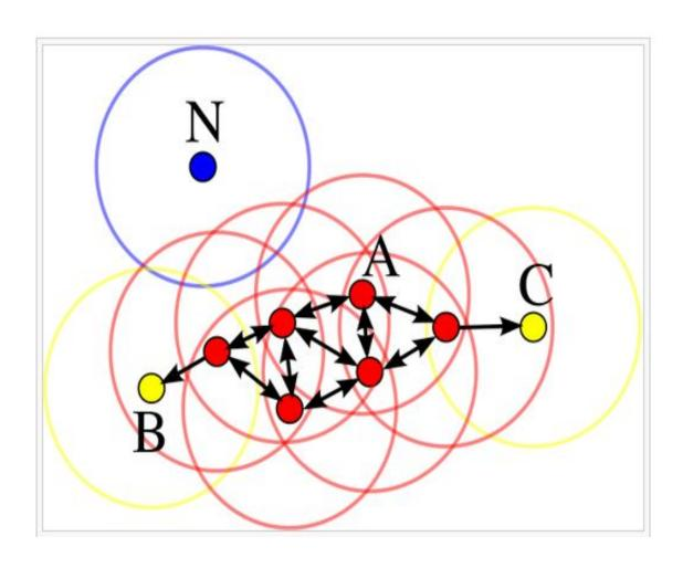
In this diagram, minPts = 3. Point A and the other red points are core points, because at least three points surround it in an  $\varepsilon$  radius. Because they are all reachable from one another, they form a single cluster. Points B and C are not core points, but are reachable from A (via other core points) and thus belong to the cluster as well. Point N is a noise point that is neither a core point nor density-reachable.
