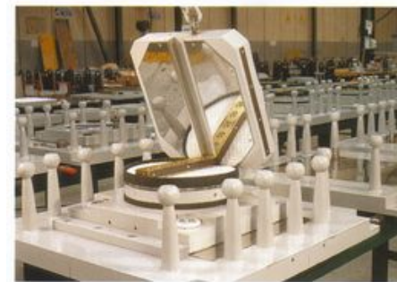
► Tuy Medio-Caracas railway (Venezuela) - 3.000 kN to 25.000 kN steel hysteresis
