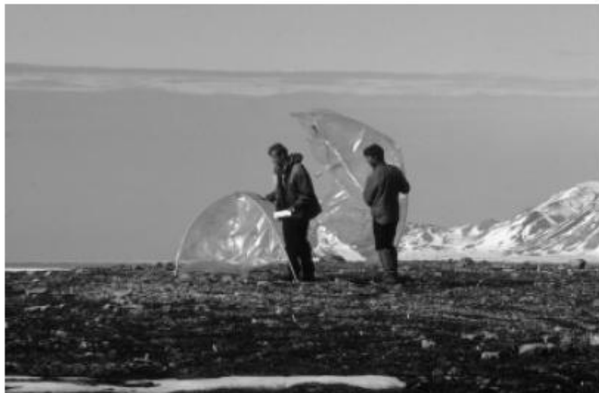
Field biologists erecting cloches for experimental warming of Arctic tundra arthropods near Ny-Åle sund.
