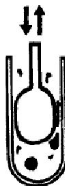
Figure 5 Schematic of pestle and tube action.
