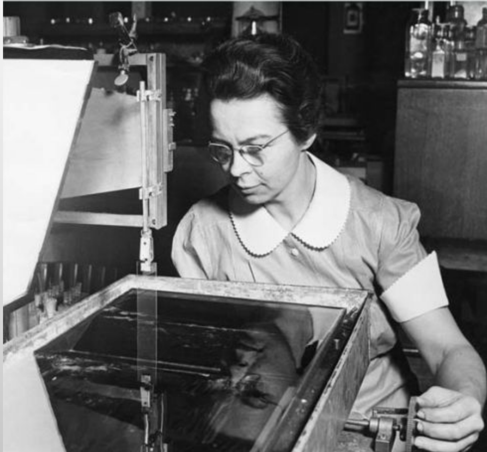
Figure 4. Katharine Blodgett (1898–1979), photographed in 1938, demonstrates an early version of the Langmuir–Blodgett trough. Turning a hand pulley repeatedly dips the glass slide into a solution of fatty acids on the surface of a water bath. The dips coat the glass with successive monolayers. (Image from the Smithsonian Institution Archives.)
