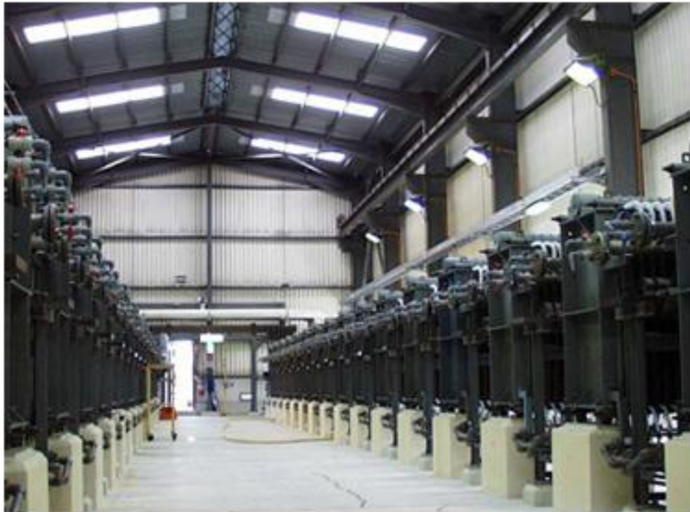
Industrial chlorine production from electrolysis of brine
