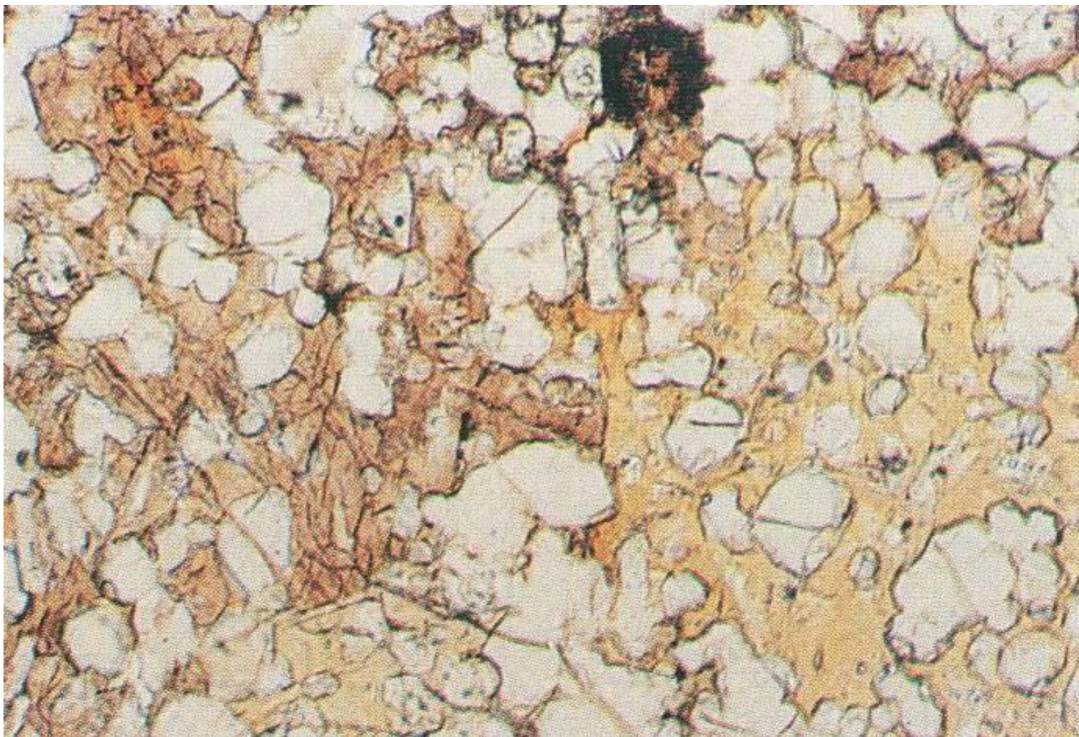
Leucite richterite lamproite, Endlich Hill, Leucite Hills, Wyoming. Resorbed fresh phenocrysts of leucite (colorless) are poikilitically enclosed by titanian potassium richterite showing yellow-to-brown pleochroism. Field of view 0.6 mm.
