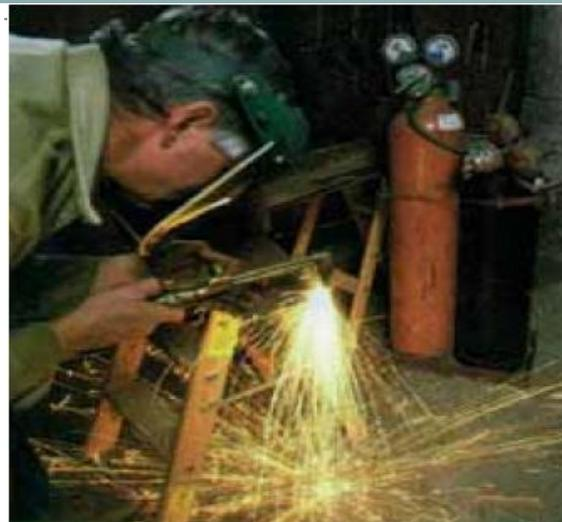
*Acetylene is used for welding with  $\text{O}_2$ . At  $3300^{\circ}\text{C}$  two metals can be welded to each other.*
