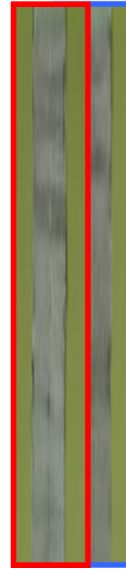
Fig13. The photograph of glass tape after a combustion rate examination
