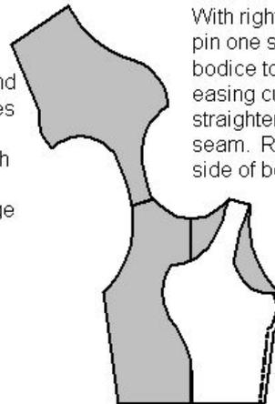
With right sides together, pin one side of front of bodice to back of bodice, easing curved front to straighter back. Sew seam. Repeat with other side of bodice.
