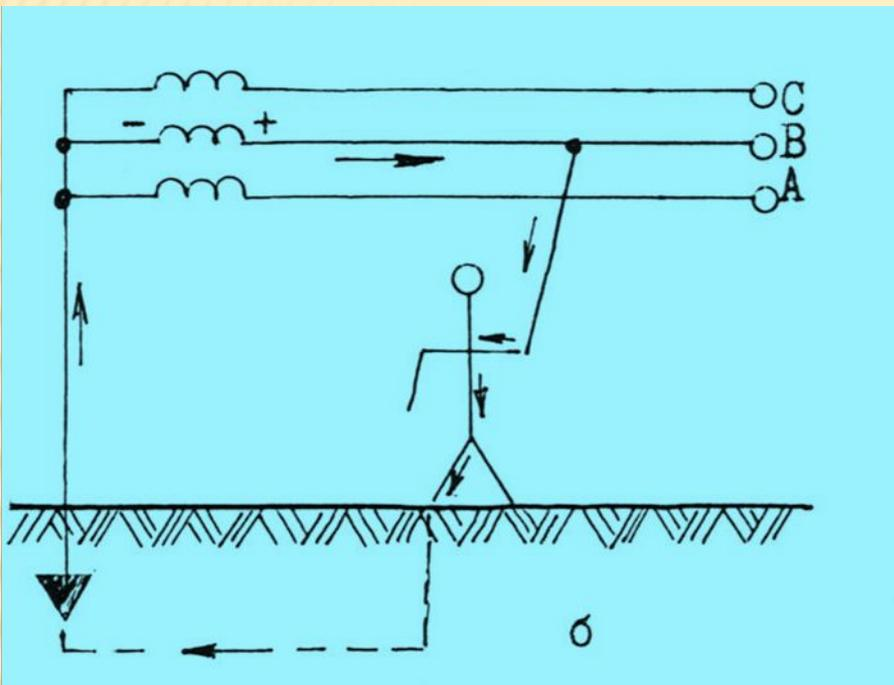
$$I_h = U_{\phi.} / (R_{h.} + R_{oc.} + R_{об.} + R_o)$$
