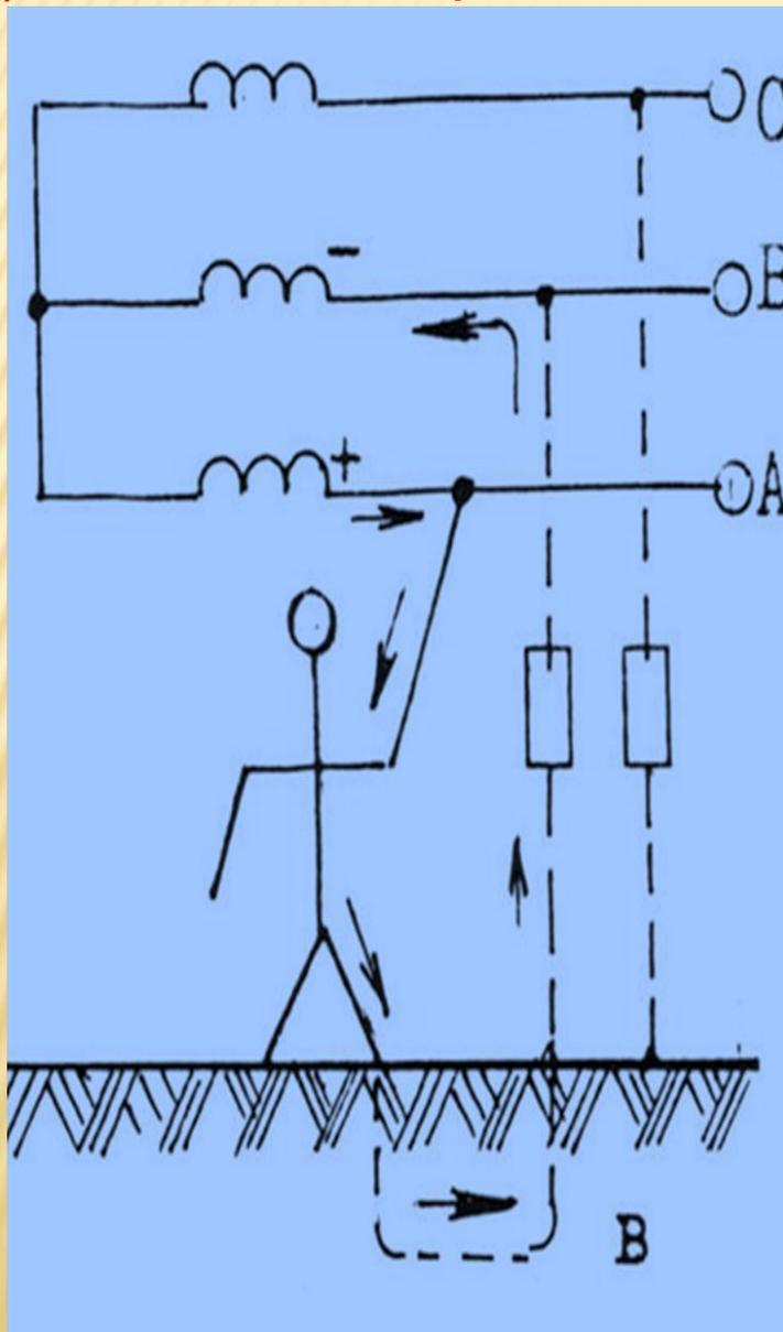
$$I_h = U_{\phi} / (R_h + R_{ос} + R_{об} + R_{из}/3)$$
