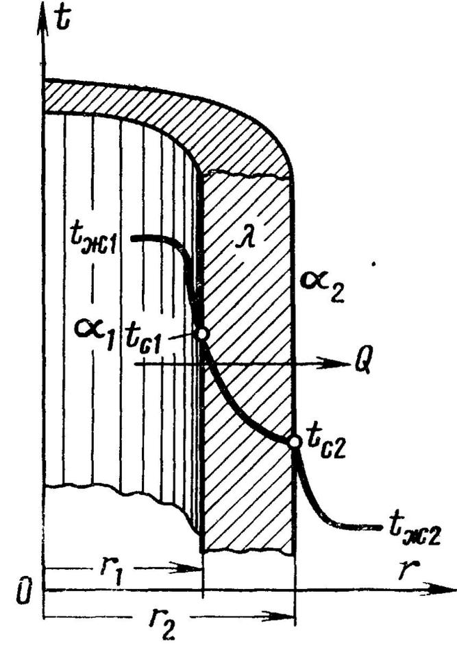
$$t_{\text{ж1}} - t_{\text{ж2}} = \frac{q_l}{\pi} \left( \frac{1}{\alpha_1 d_1} + \frac{1}{2\lambda} \ln \frac{d_2}{d_1} + \frac{1}{\alpha_2 d_2} \right)$$
