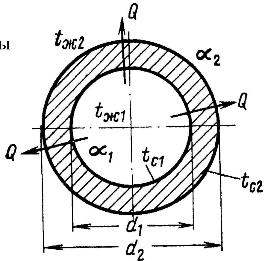
$$Q = \frac{\pi(t_{ж1} - t_{ж2})}{\frac{1}{\alpha_1 d_1^2} + \frac{1}{2\lambda} \left( \frac{1}{d_1} - \frac{1}{d_2} \right) + \frac{1}{\alpha_2 d_2^2}} = k_{ш} \pi (t_{ж1} - t_{ж2})$$
