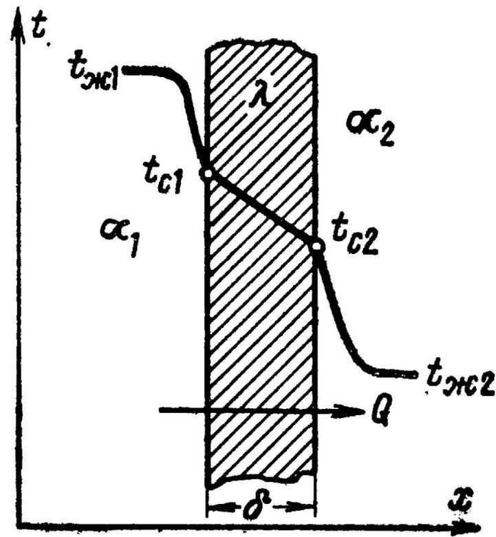
$$q = \frac{1}{\frac{1}{\alpha_1} + \frac{\delta}{\lambda} + \frac{1}{\alpha_2}} (t_{ж1} - t_{ж2}) = k(t_{ж1} - t_{ж2})$$
