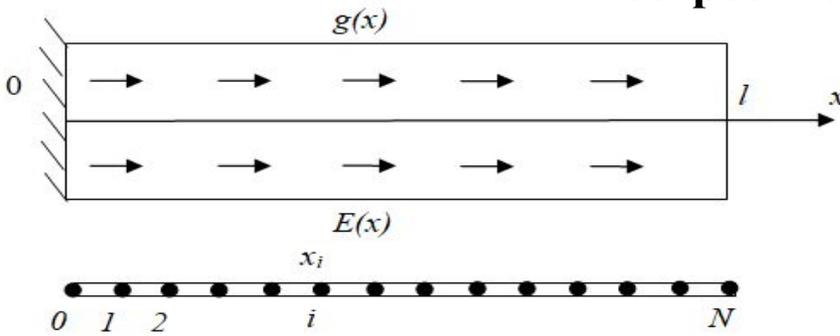
$\bar{\omega} = \{x_i = ih, \quad i = \overline{1, N}, \quad h = l/N\}$
