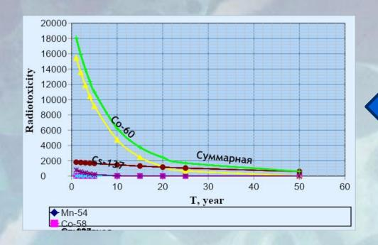
The contribution of each element in the change over time in the water radiotoxicity of SRW at the KhNPP formed in 2011.
