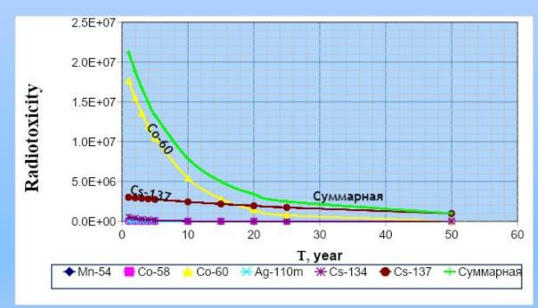
The changing of total radioactivity of the SRW during storage time **in the air** at the KhNPP formed in 2011.
