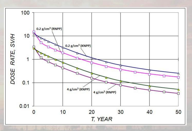
The changes in dose rate (in relative units) and the flux of gamma rays **depend on** the storage time and density of SRW 0.2 g/cm<sup>3</sup> at the KhNPP and RNPP
