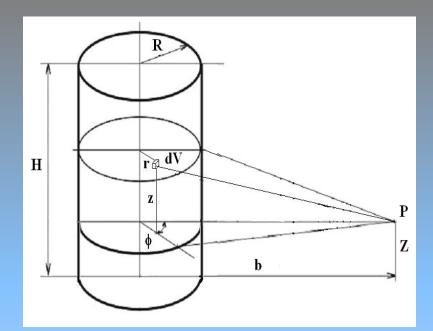
The geometrical demensions of a cylindrical volume source.
