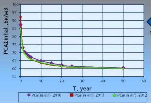
The changing of the concentration of the radionuclides mixture in the air over time at KhNPP during 2010-2012.
