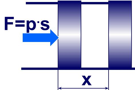
$$\begin{aligned} E_k &= T \cdot x = F_i \cdot x \\ &= m \cdot a \cdot x = m \cdot v/t \cdot x \\ &= v/2 \cdot t = mv^2/2 \end{aligned}$$
