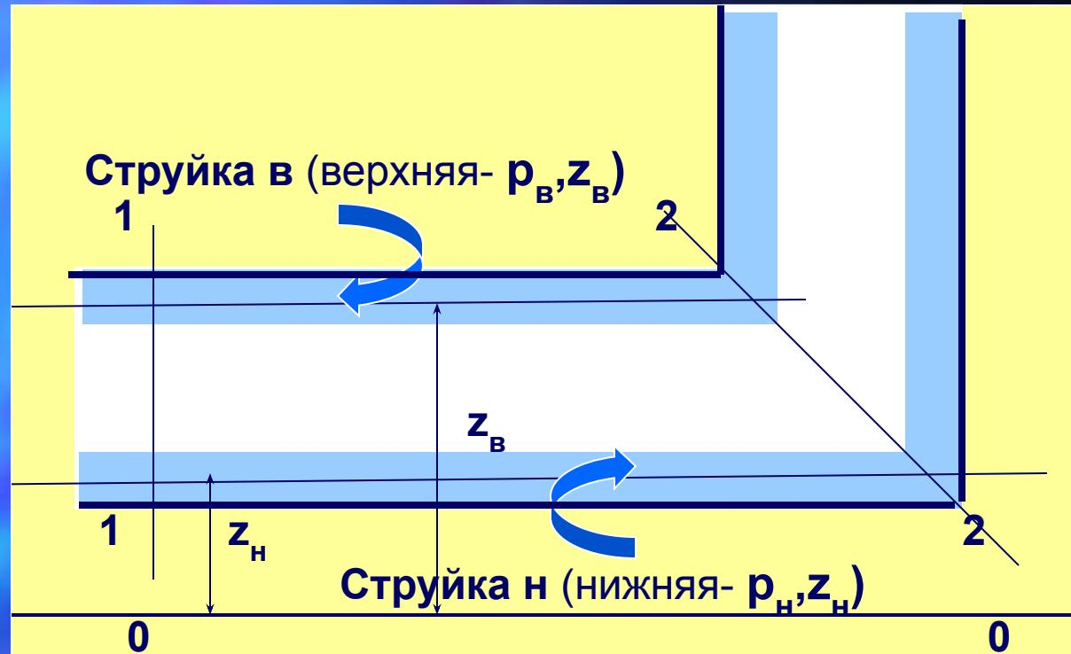
$$\begin{aligned} E_p &= \int dm(gz + p/\rho) = \int dm(gz + p/\rho) = \\ &= mgz + mp/\rho \end{aligned}$$
