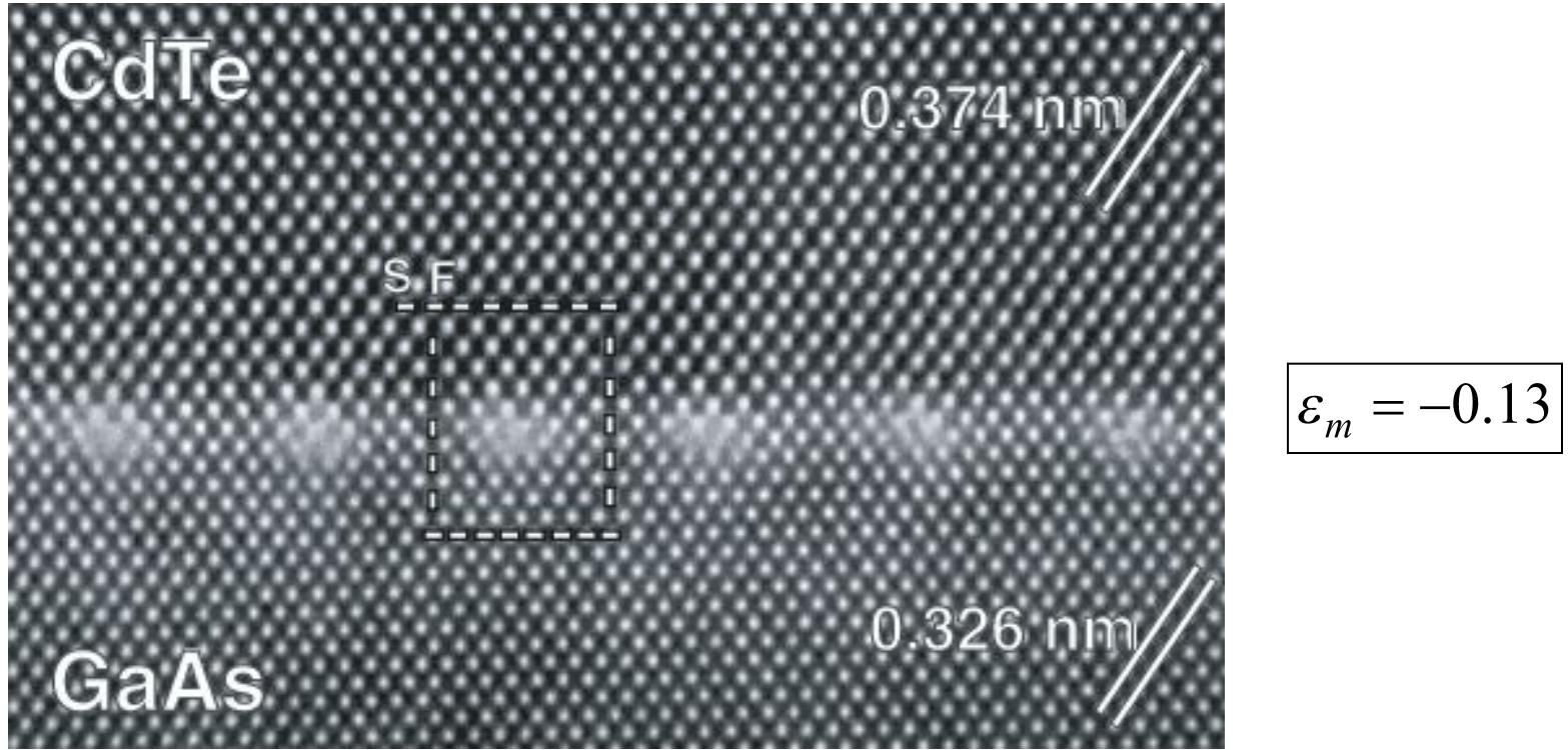
Atomic resolution transmission electron micrograph of an interface between CdTe and GaAs where the misfit strain is relaxed by the introduction of edge dislocations. The letters 'S' and 'F' refer to 'start' and 'finish' for the Burgers circuit around the dislocation. The bright white spots correspond to atomic positions and the fuzzy white clusters at the interface correspond to the cores of the dislocations. After Schwartzman and Sinclair (1991).
