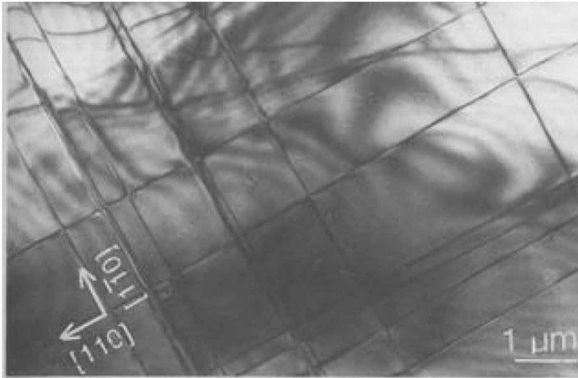
A plan-view, bright-field transmission electron microscopy (TEM) image of misfit dislocations within the interface between a 200-nm thick  $\text{Si}_{0.9}\text{Ge}_{0.1}$  film and a much thicker (001) Si substrate. The dislocations form a crossed-grid pattern which is oriented along two  $<110>$  directions on the (001) interface plane. After Fukuda et al. (1988).
