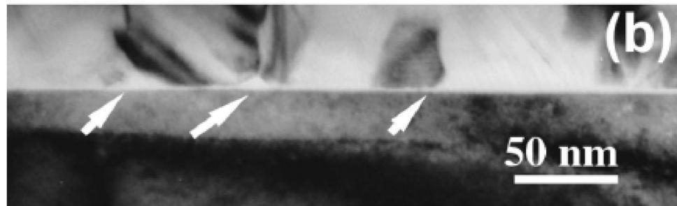
Cross-sectional bright-field TEM micrographs of a GaAs/GaN hetrostructure. Vertical black arrows show the directions in the zinc blende and wurtzite lattices. A horizontal black arrow marks the location of the heterointerface. White arrows indicate nanocavities located in the GaAs layer near the interface. Chaldyshev et al. 2005
