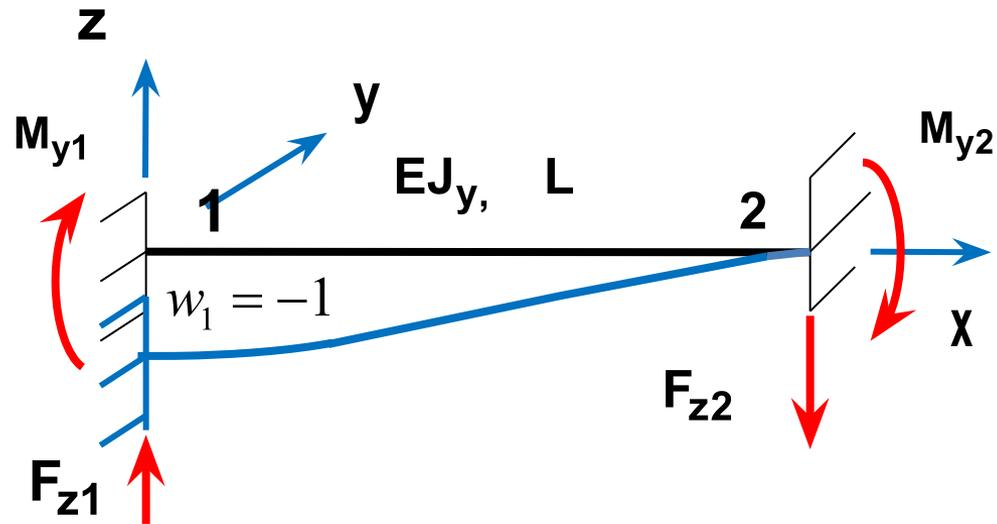
$$w_2(L) = 0 \quad \frac{M_{y1} * L^2}{2EJ_y} + \frac{F_{z1} * L^3}{6EJ_y} = -1 \quad \rightarrow \quad F_{z1} = \frac{12EJ_y}{L^3}$$
