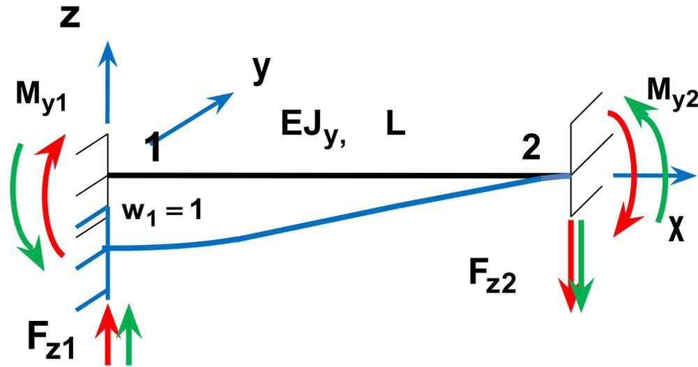
$$F_{z1} - F_{z2} = 0 \quad F_{z2} = \frac{12EJ_y}{L^3} \quad \longrightarrow \quad F_{z1} = \frac{12EJ_y}{L^3} \quad \longrightarrow \quad F_{z2} = -\frac{12EJ_y}{L^3}$$
