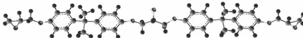
The formula and model of epoxy molecule
