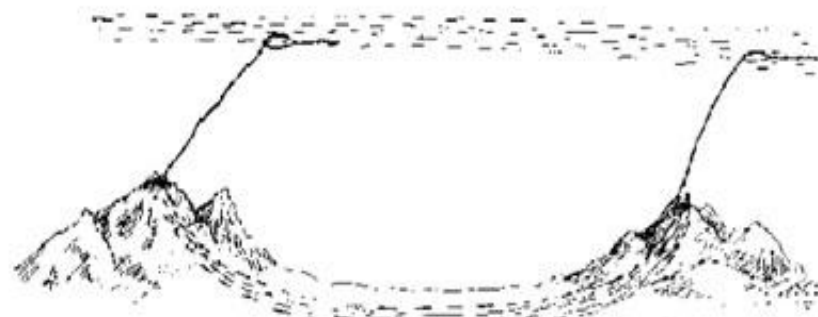
Cohasset Mountain No. 19 miles apart Coaranda 1866 Spur of Blue Ridge Spur of Blue Ridge Short signals by Morse's telegraph. Later in this station by kite on each mountain, consisting of which was a small copper wire, attached to cabinets and ground with string in water. The signals passed during the cloudy part of the day. Estimated about fifty hundred feet.
