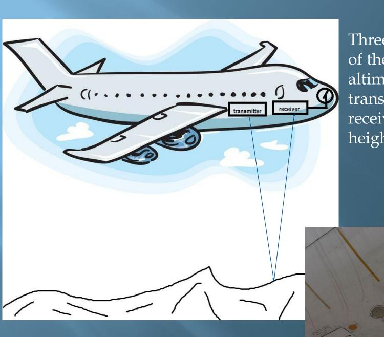
Three main parts of the radio altimeter are: transmitter, receiver and height indicator
