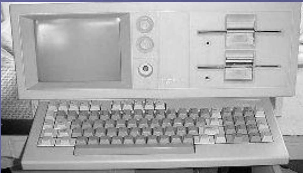
HYPERION 8088 portable boxtop 5 inch CRT display, 300 k ram, dual 360K floppys
