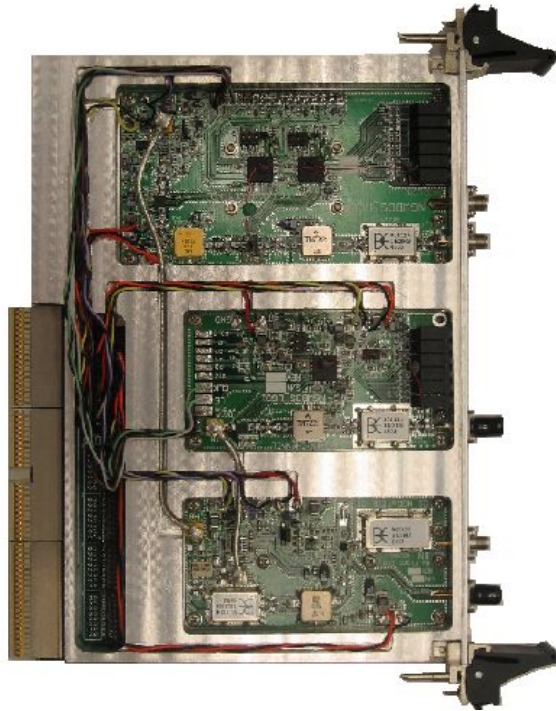
Compact PCI module (9" x 6.5" x 1")
